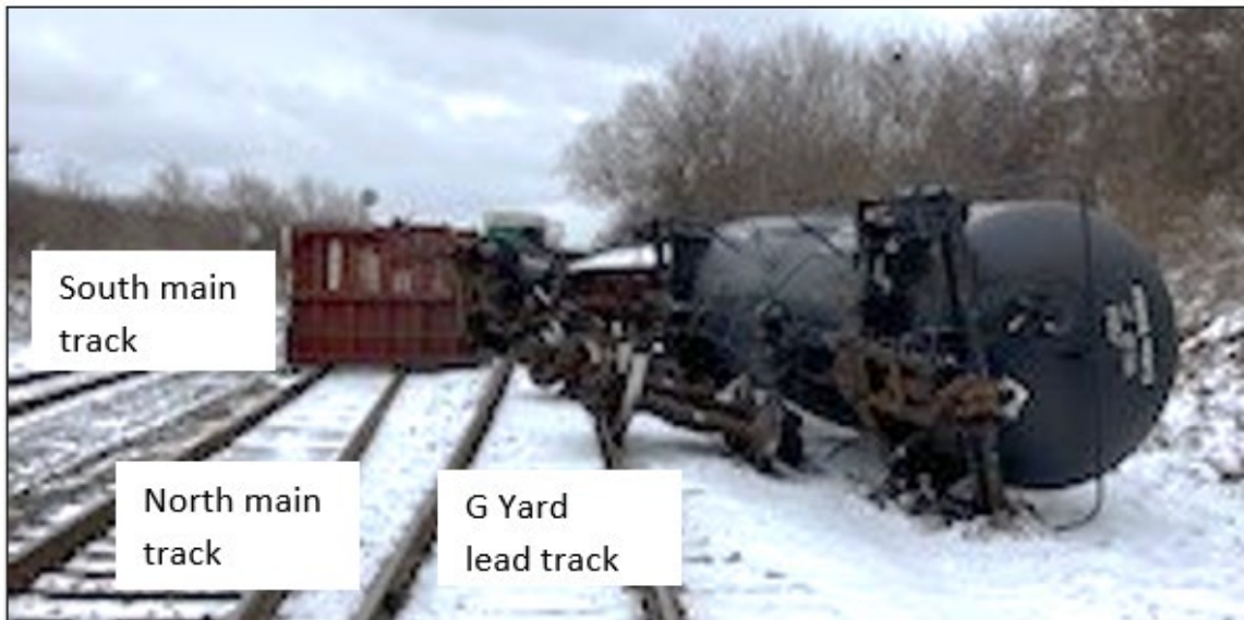
Figure 3. Occurrence location, looking west, showing the first 2 derailed cars at the split switch derail, including a box car foul of the main track (Source: Canadian Pacific, with TSB annotations)
