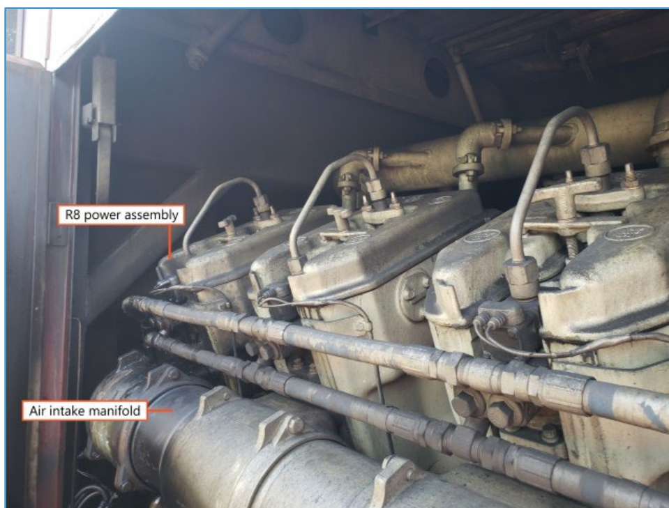
Figure 4. Air intake manifold and R8 power assembly on locomotive CP 9779 (Source: TSB)
