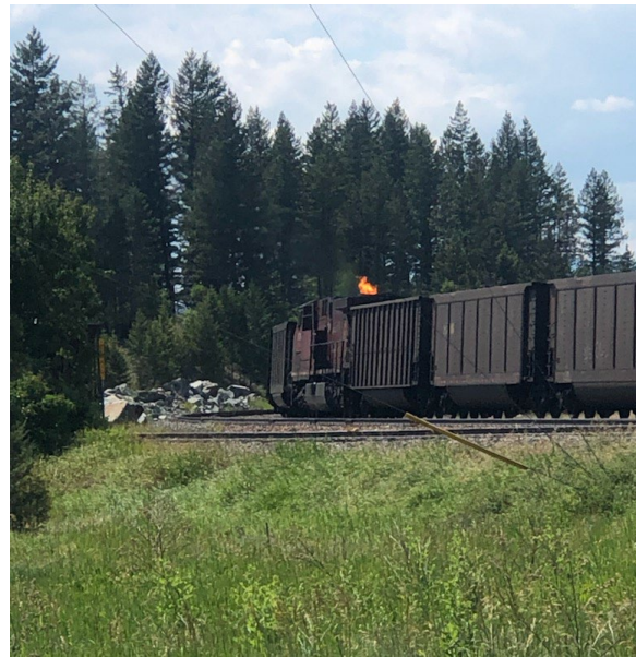
Figure 2. Exhaust stack fire on the mid-train remote locomotive (Source: Elko resident)
