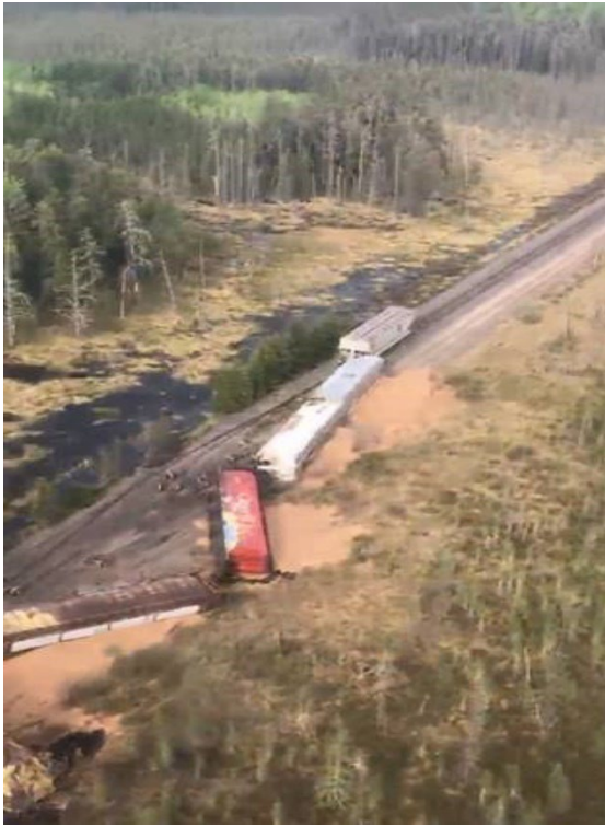
Figure 4. Water accumulation beside the north track (Source: Canadian Pacific)
