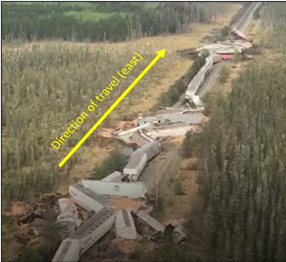
Figure 2. Occurrence site showing the 2 pile-ups of derailed cars (Source: Canadian Pacific, with TSB annotations)
