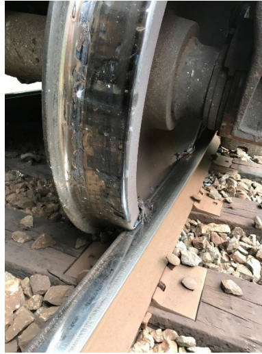
Figure 4. L4 wheel of car CNPX 3373 derailed inside the track gauge of the south rail (Source: Canadian National)
