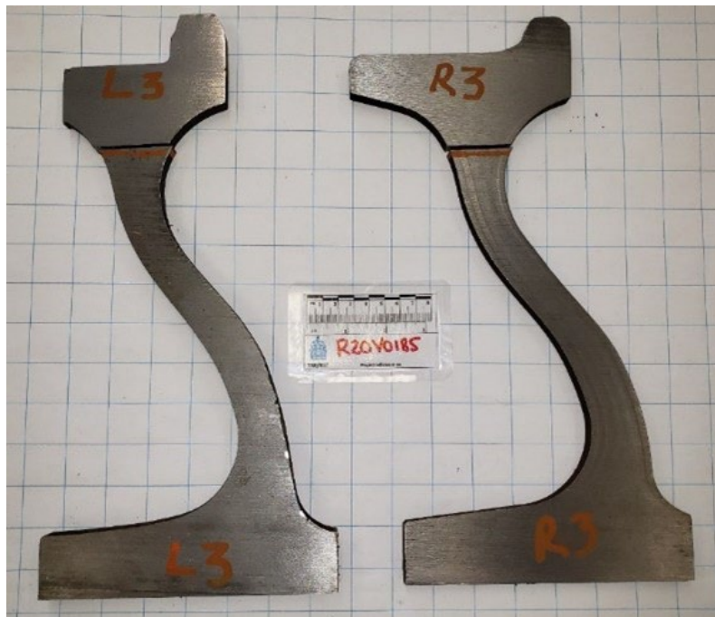
Figure 25. Radial samples from the L3 wheel (on the left) and R3 wheel (on the right) sent for X-ray diffraction analysis (Source: TSB)
