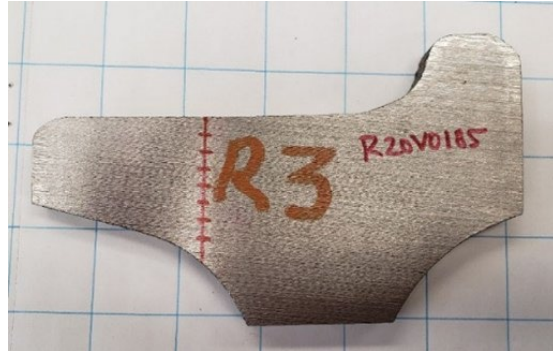
Figure 27. Residual stress measurement locations for the R3 wheel section (Source: TSB)
