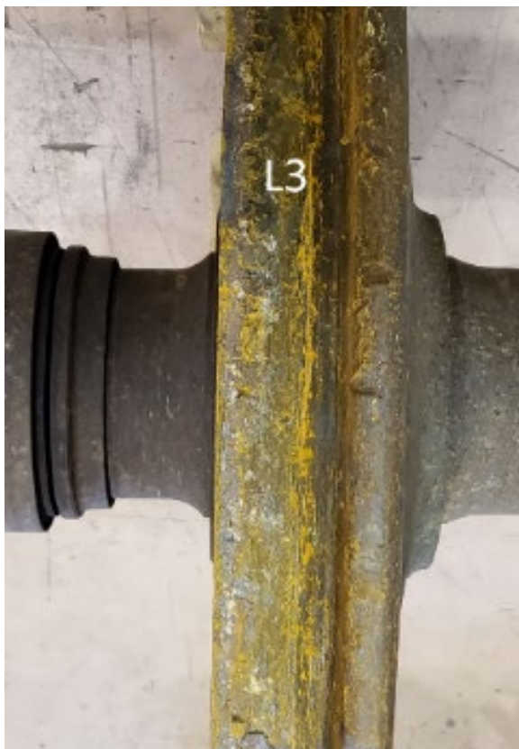
Figure 20. Condition of the L3 wheel after the derailment, with its rim width reduced by 1.75 inches (Source: TSB)
