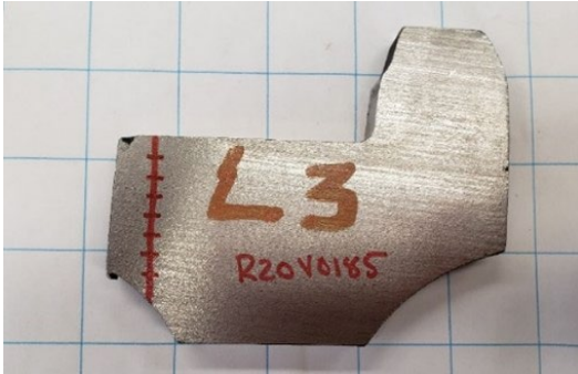
Figure 26. Residual stress measurement locations for the L3 wheel section (Source: TSB)
