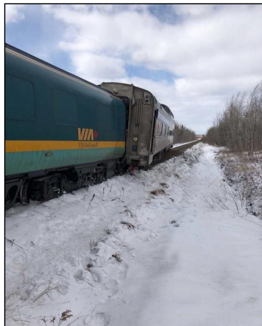
Figure 3. The last 2 VIA passenger cars, derailed upright (Source: Canadian National Railway Company)
