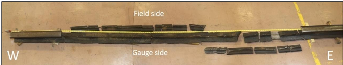
Figure 11. Recovered rail fragments (Source: TSB)
