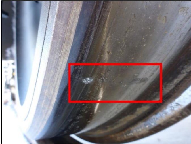
Figure 6. Impact mark on wheel of the 10th car (Source: TSB)
