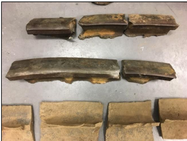
Figure 12. Fragments of recovered rail (Source: TSB)
