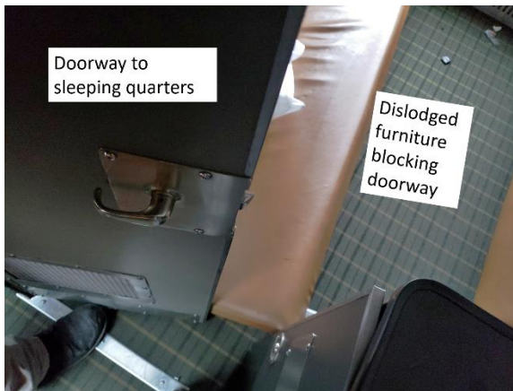
Figure 7. Blocked doorway on VIA 8711 (Source: TSB)
