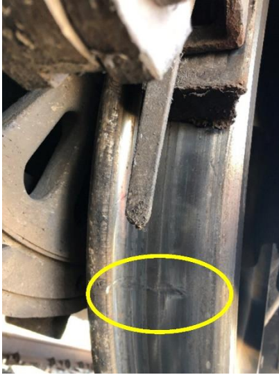
Figure 3. Scuff mark on the tread of wheel L5 on the lead locomotive (Source: TSB)
