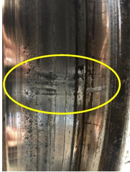
Figure 4. Scuff mark on the tread of wheel L6 on the lead locomotive (Source: TSB)
