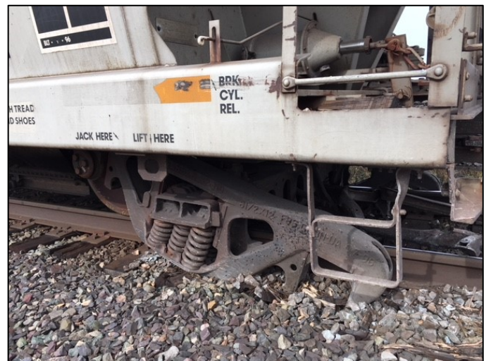
Figure 3. Car CEFX 350816 with number 1 axle and wheels missing (Source: CN)
