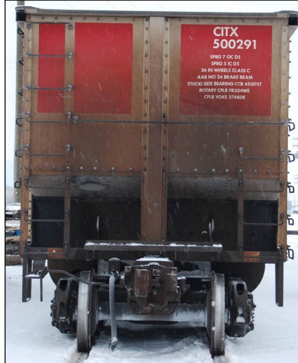
Figure 6. Aluminum gondola coal car with rotary coupler (Source: TSB)
