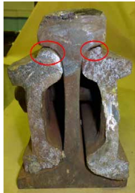
Figure 3. East-end view of the south rail joint. Signs of fatigue are circled in red.
