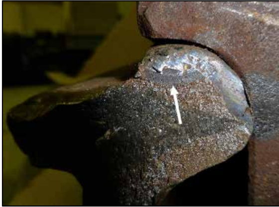
Figure 4. Gauge-side joint bar with fatigue identified by arrow
