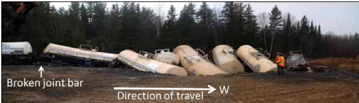
Figure 2. Tank cars derailed in various positions
