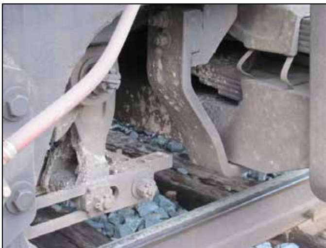
Photo 2. Mud on the underside of the lead locomotive
