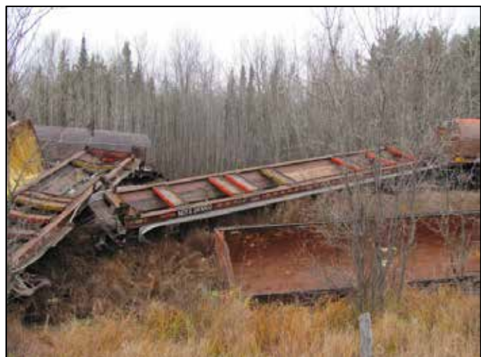
Photo 4. Additional derailed empty covered gondola cars
