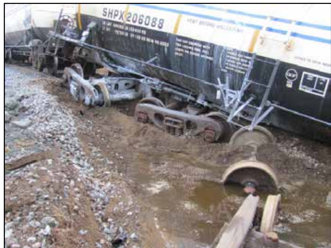
Photo 3. Derailed cars and appliances partially submerged
