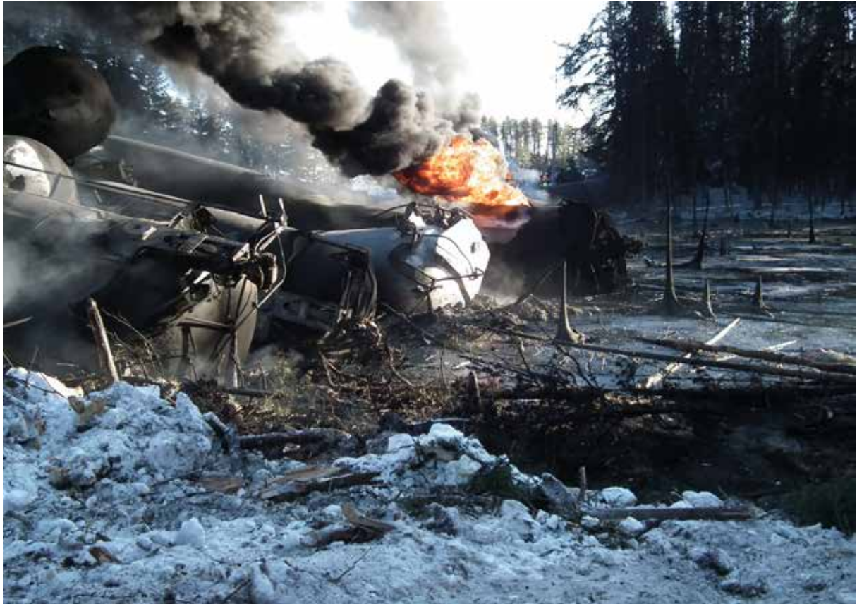
Photo 2. Derailment site with tank car burning from thermal tear (16 February 2015)
