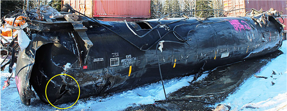
Photo 5. Puncture to tank GATX 200483
