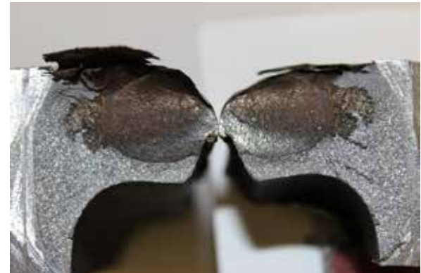
Photo 11. Transverse defect found in rail piece No. 2
