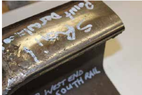
Photo 7. Head checks and shelling on rail piece No. 2
