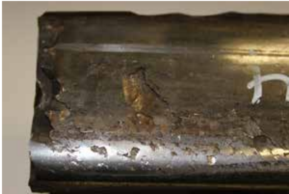
Photo 6. Head checks and shelling on rail piece No. 1
