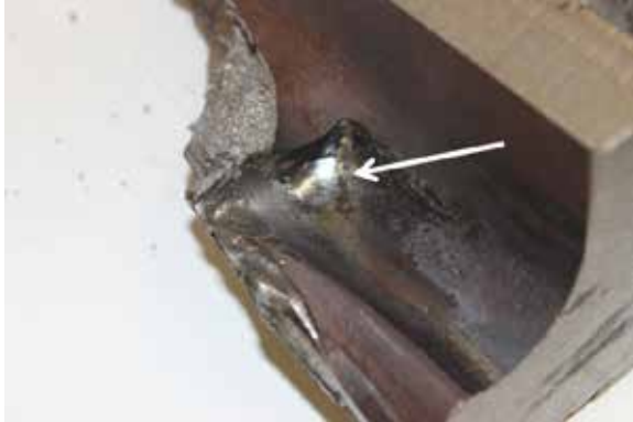
Photo 4. Deformation from joint bar contact at the fillet under the head on the gauge side of rail piece No. 1 (arrow)
