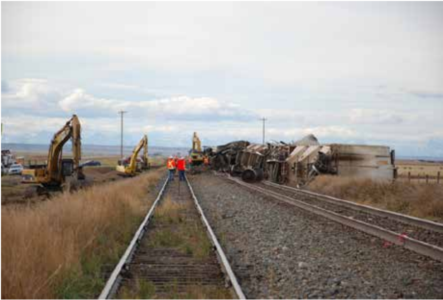
Photo 1. Derailed cars on the main track, showing storage track on left (looking west)
