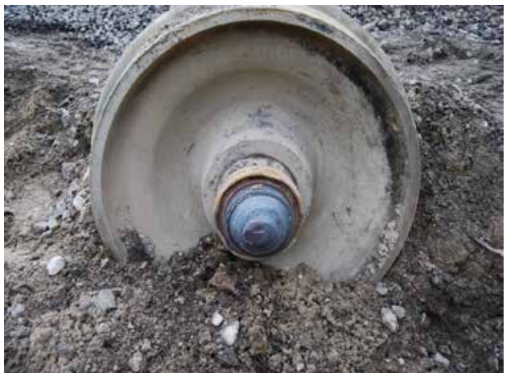
Photo 2. DTTX 680968 L3 wheel and burnt-off axle journal
