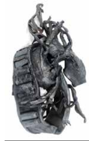
Photo 6. Outboard cone assembly
