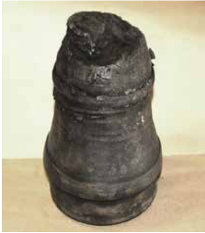
Photo 4. Failed burnt-off axle journal stub
