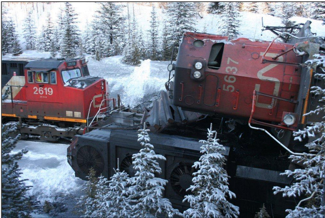
Photo 1. Lead locomotive (CN 5637) positioned on top of the 3rd locomotive
