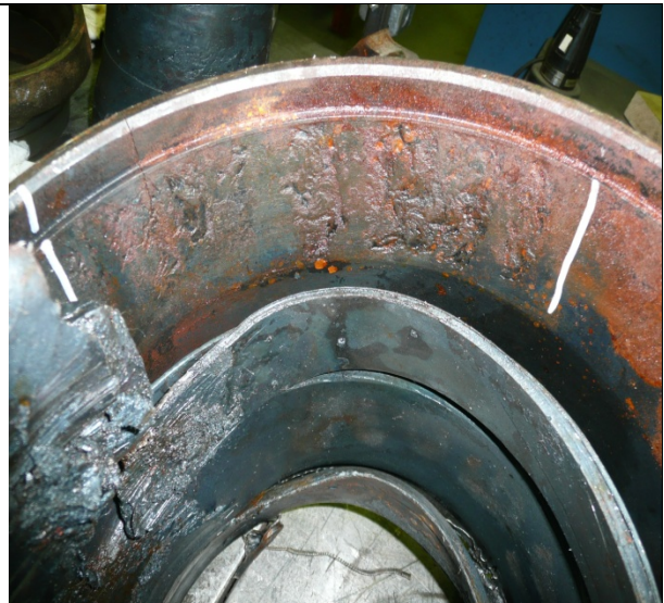
Photo 3. L-4 spalled inboard cup path (typical)
