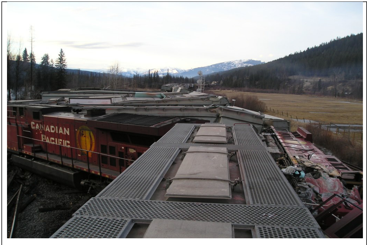
Photo 1. Derailment damage of cars from train 300 and train 671
