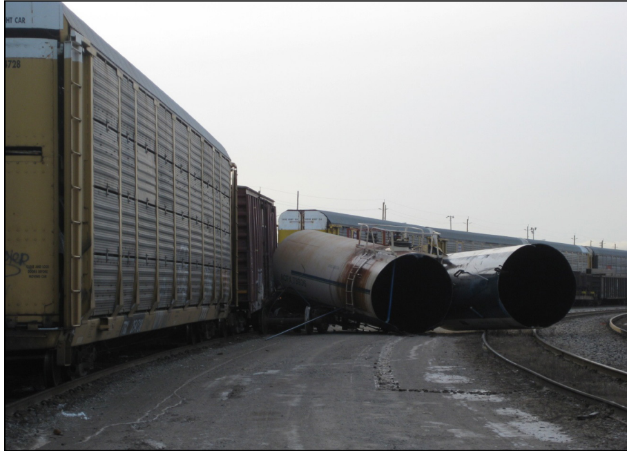
Photo 1. ACFX 73936 fractured and derailed
