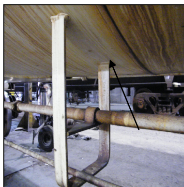
Photo 3. Location of fracture origin (ACFX 73937)
