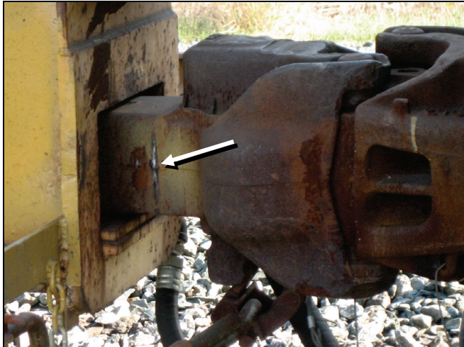
Photo 2a. Severe gouging on the side of the coupler shank of car BGSX 122226
