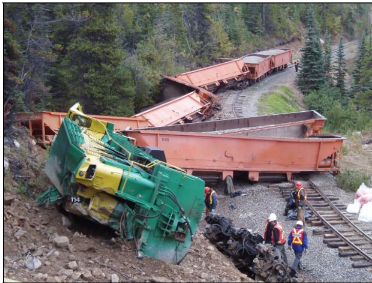
Photo 1. Derailment of work train
