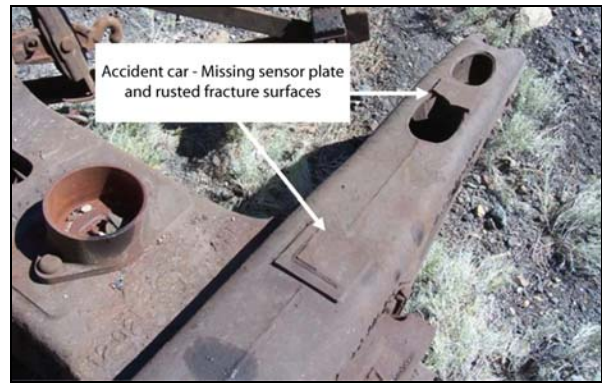
Photo 13. Accident car with missing sensor plate (Source: Canadian National)
