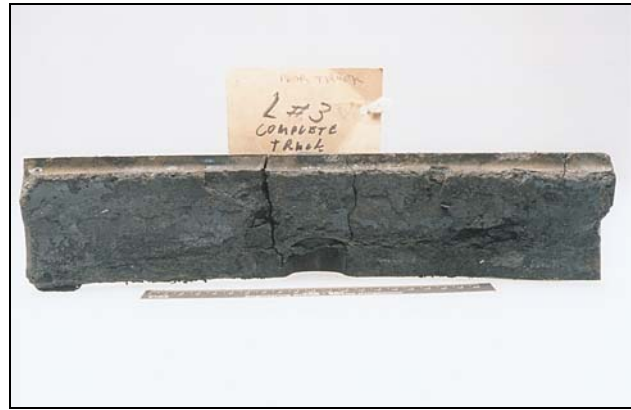
Photo 11. Inboard face of the locomotive brake shoe
