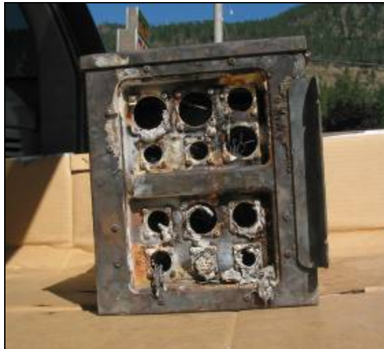
Photo 8. Burnt locomotive event recorder
