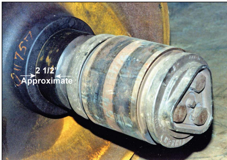
Photo 3. Wheel movement on axle seat (2 ½ inches), typical of loose wheel-related occurrences
