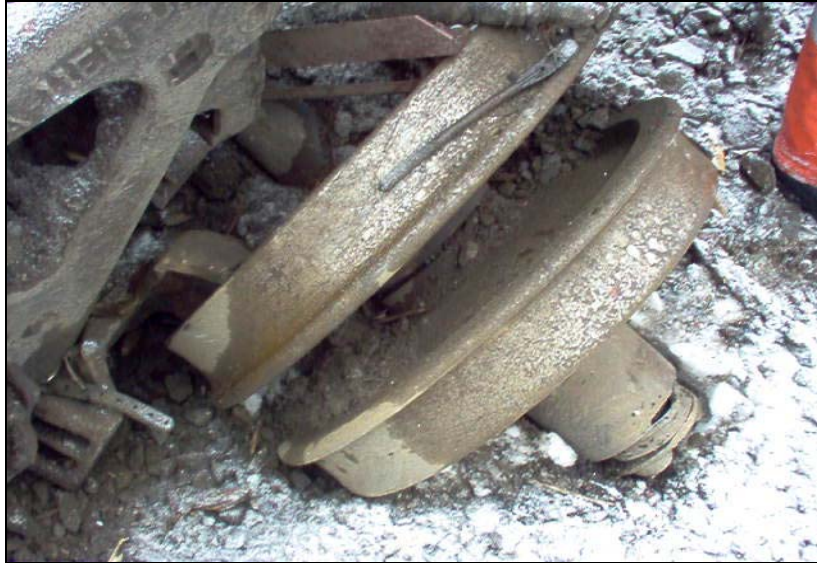
Photo 1. No. 1 wheel set from car CP 346875 (Source: Canadian Pacific Railway)
