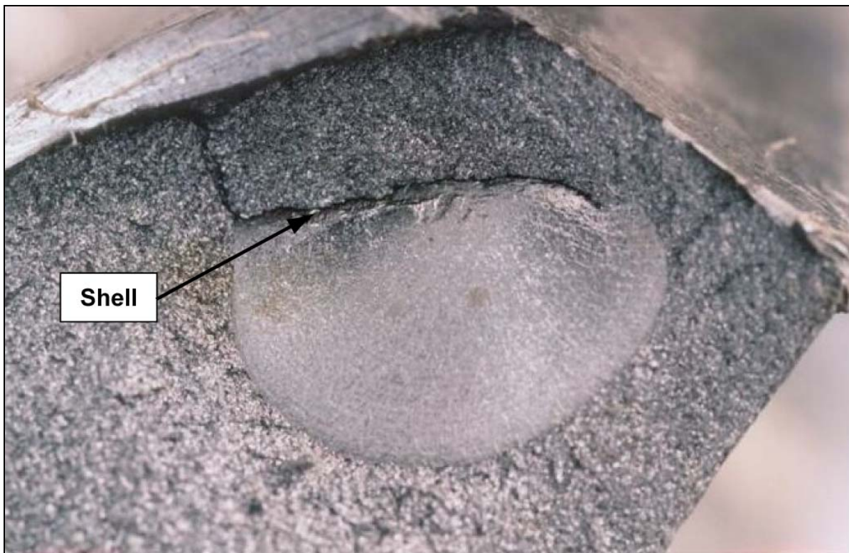
Photo 2. Close-up of detail fracture
