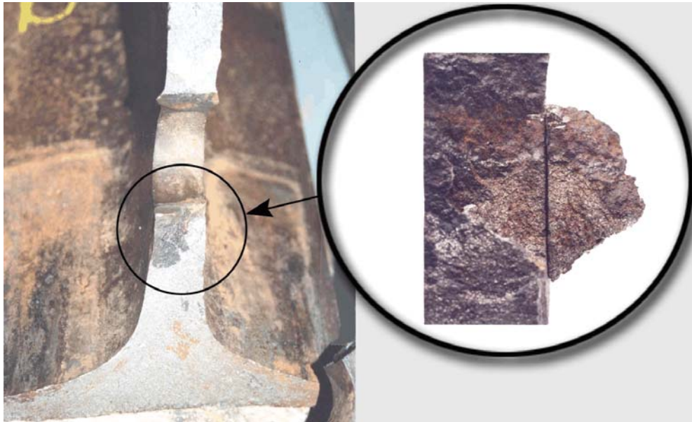
Photo 2. Pre-crack in third bolt hole. Exploded view is a close-up of the full pre-crack fracture surface with the mating surface removed.
