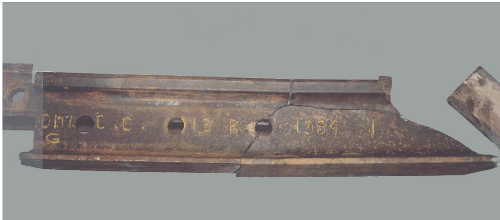
Photo 1. Reconstructed rail from suspected POD
