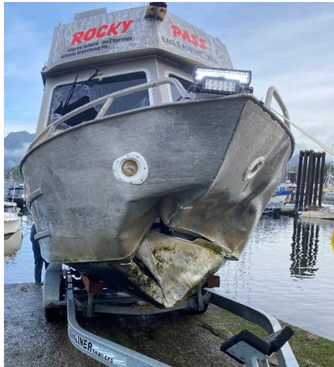
Figure 2. Damage sustained by the Rocky Pass following the occurrence (Source: Royal Canadian Mounted Police)
