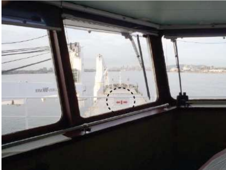
Photo 5. View from centreline of BBC Steinhoeft sister vessel showing the centreline marker (within the dashed circle).
