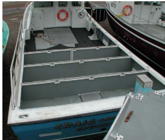
Photo 2. Working deck with transverse pound boards (Courtesy of Briand Marine Surveys)
