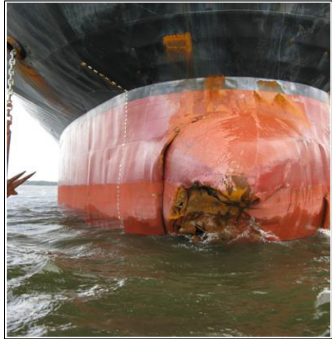
Photo 5. Damage to the bulbous bow.
