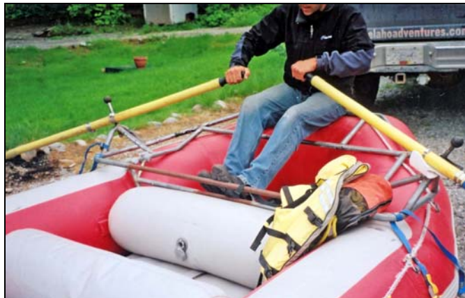
Photo 1. Stern view showing the steering frame with oars clipped to thole pins. Indicates the position of the trip leader and the transverse buoyancy chambers.
