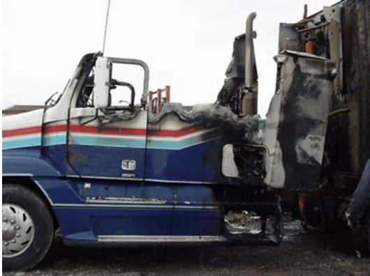
Tractor fire damage
