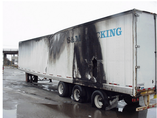
Drop trailer fire damage
