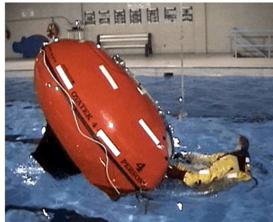
Photo 5. Ovatek 4: trim while boarding during TSB pool tests
