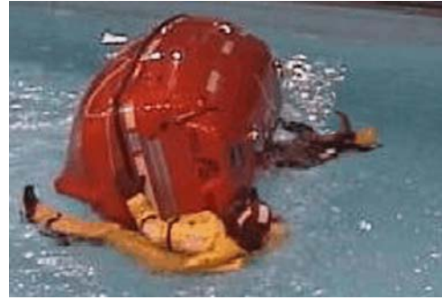
Photo 4. Swamped Ovatek 7 on its side during TSB pool tests
