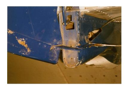
required 36 pounds of steady pull on the trailing edge of the rudder to break the rudder out of its jammed position. This steady pull of 36 pounds equated to 180 pounds if the force was applied to the rudder pedal. However, given that the direction of cable pull tended to increase the jamming by closing the horn, it would not have been possible to break the rudder jam with the application of right rudder.
