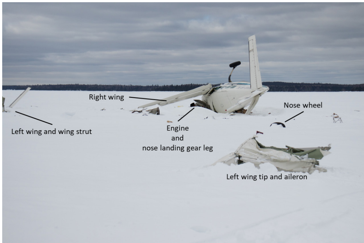
Figure 1. View along the wreckage trail (Source: TSB)
