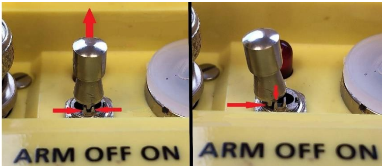
Figure 13. ELT switch locking system similar to the system in the occurrence (Source: TSB)
