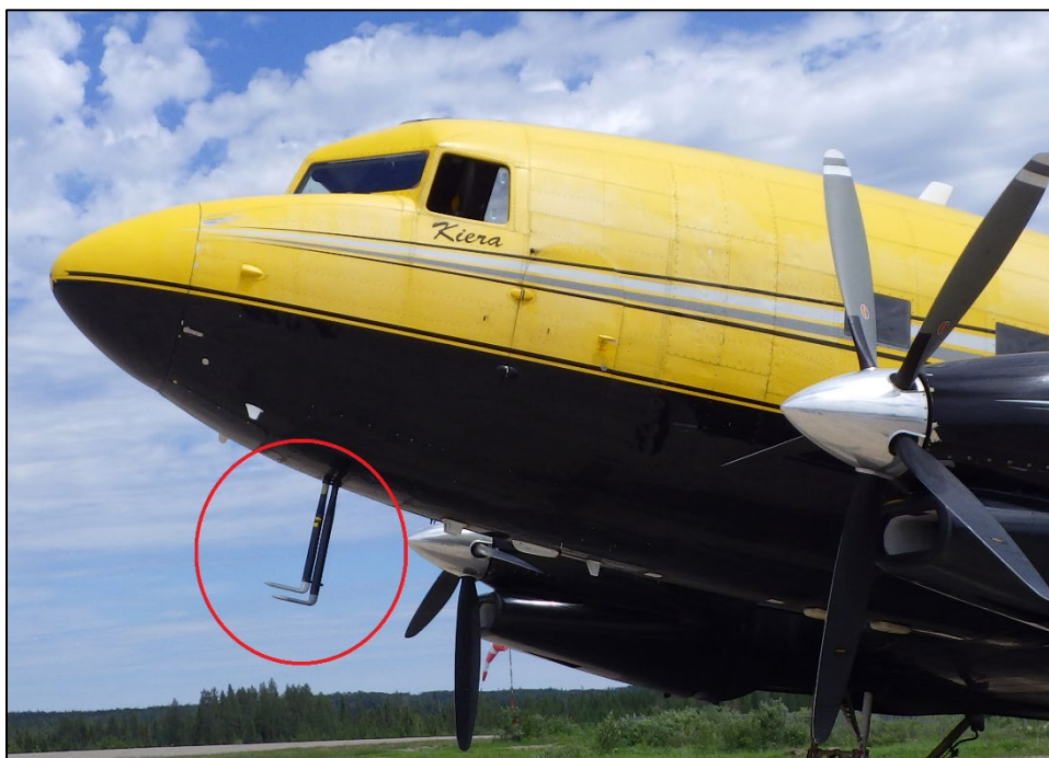
Figure 4. Pitot-static tubes on a DC3-TP67 aircraft (Source: TSB)
