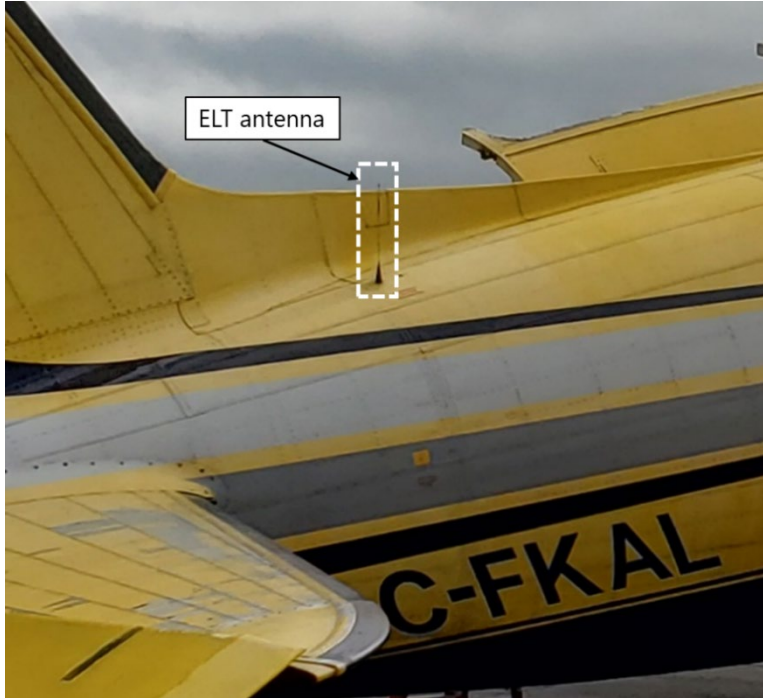
Figure 3. Photo of the occurrence aircraft emergency locator transmitter antenna location before the occurrence (Source: TSB)
