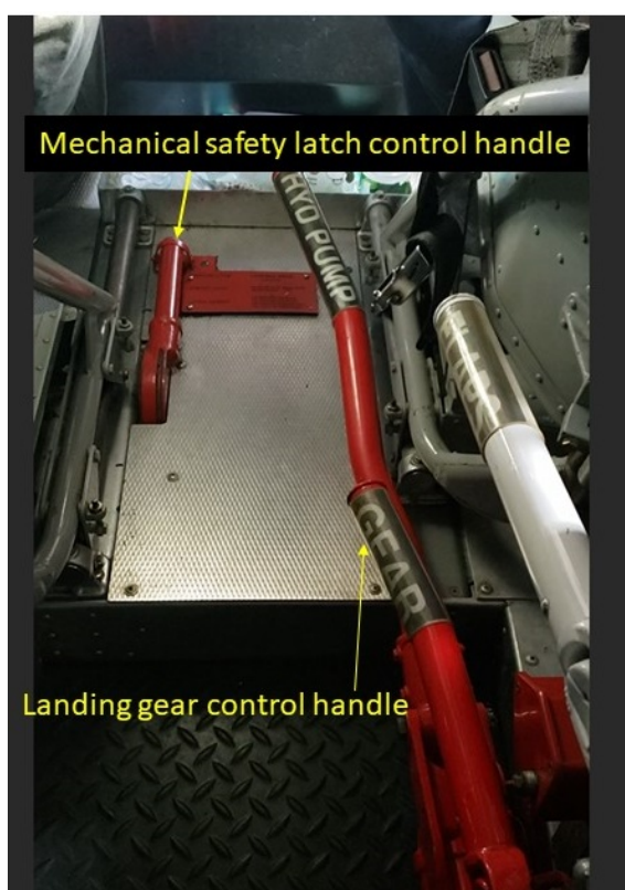
Figure 3. Main landing gear control handle and mechanical safety latch control handle (Source: TSB)
