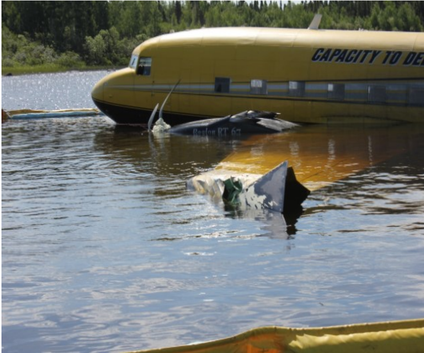
Figure 6. Occurrence aircraft's left wingtip, with crush damage (Source: TSB)
