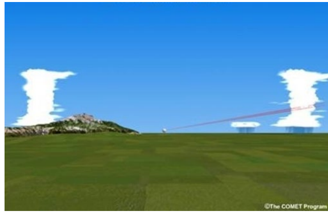
Figure 1. Schematic showing radar beams' limits of detection of precipitation (Source: The COMET Program of the University Corporation for Atmospheric Research, U.S. National Oceanic and Atmospheric Administration)
