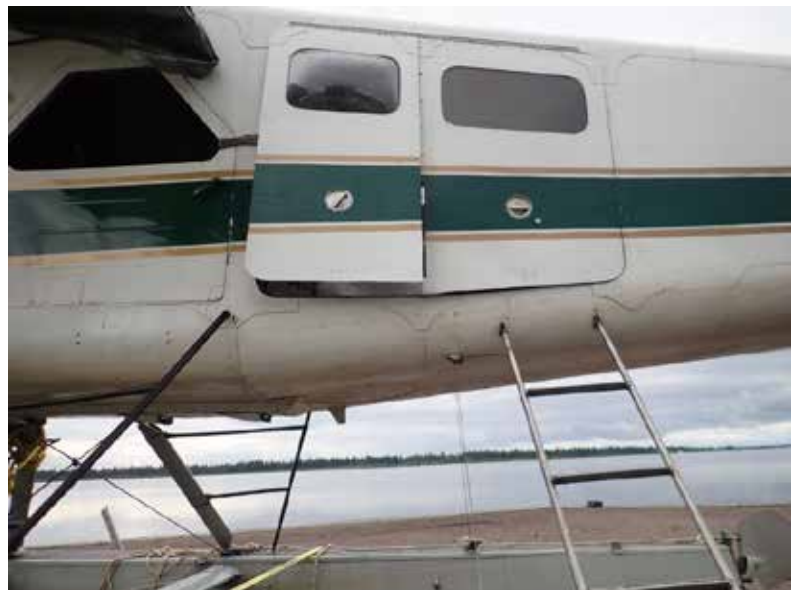
Figure 1. Alaska door on the occurrence aircraft (Source: J. Cooper)
