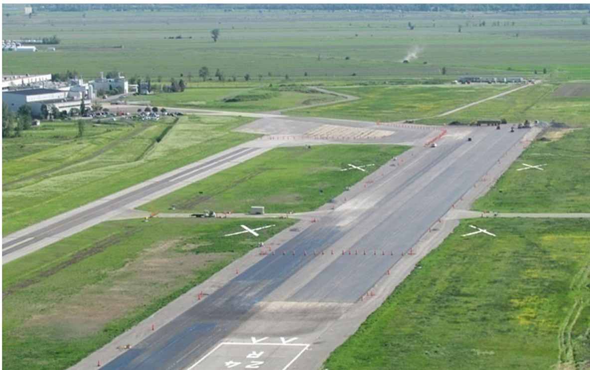
Figure 4. Marking (orange cones and white Xs) on first 2801 feet of Runway 24R, indicating completely closed portion of runway
