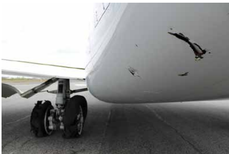
Figure 2. View of damage to left main landing gear and rear centre fuselage
