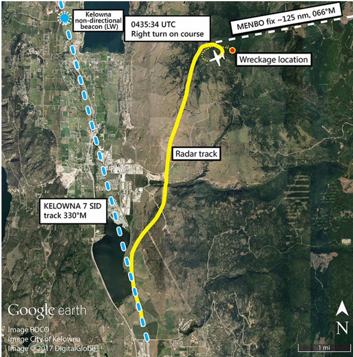
Figure 1. Overhead view of C-GTNG's flight path (Source: Google Earth, with TSB annotations)
