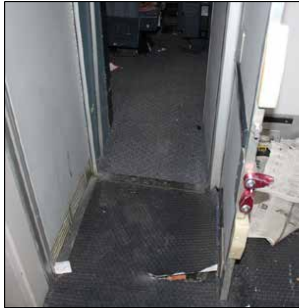
Figure 9. Floor damage aft of cockpit door
