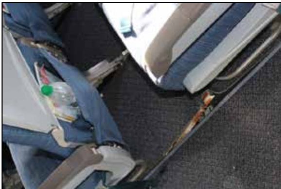
Figure 10. Floor damage forward of passenger seat 31D
