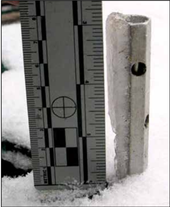
Figure 4. Ice on the outside air temperature probe
