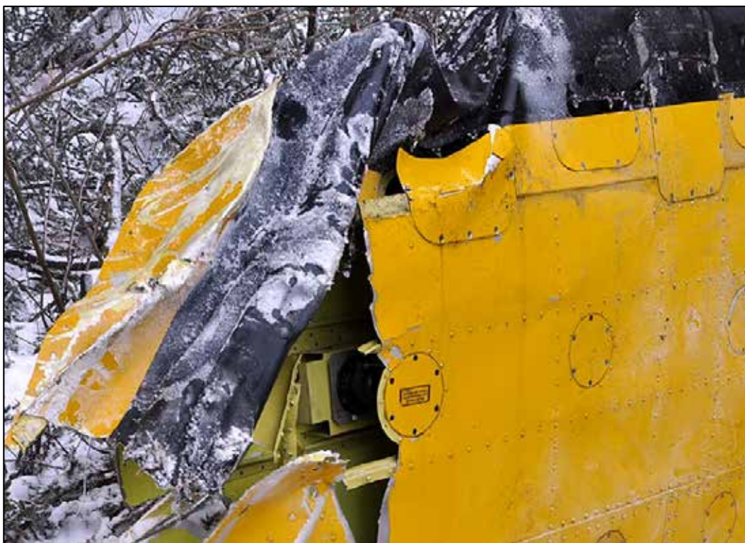
Figure 8. Ice on the leading edge of the right wing outboard section
