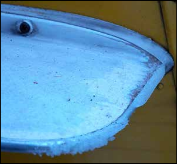
Figure 5. Ice on an antenna on the right side of the vertical stabilizer
