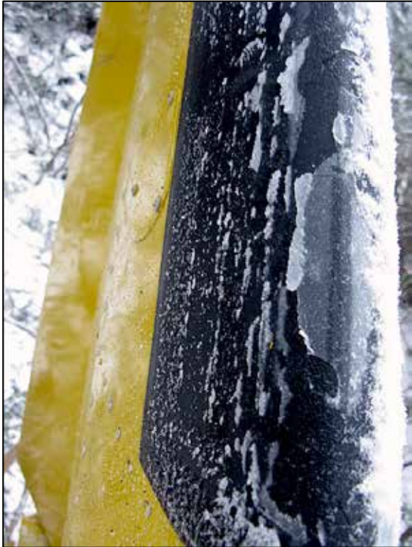
Figure 6. Ice on the right side of the vertical stabilizer
