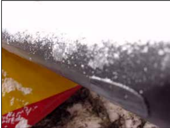
Figure 7. Ice on the leading edge of the left horizontal stabilizer
