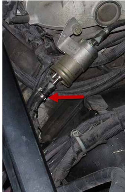
Photo 3. View showing crimped steel ring securing the connector of an identical, undamaged, belt loader
