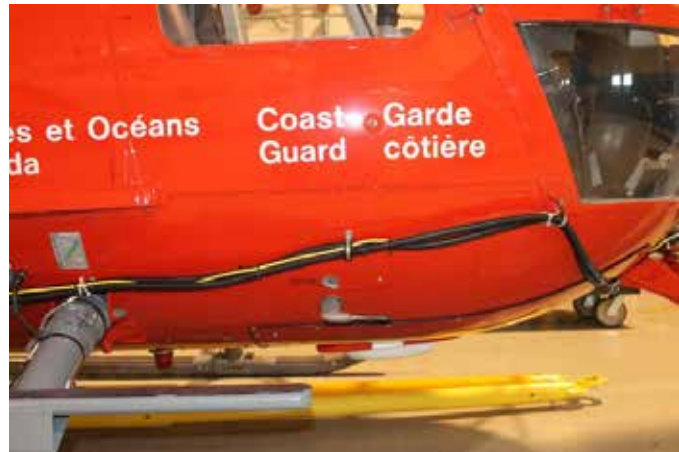
Photo 4. Example of cable bundle routing as in August 2013
