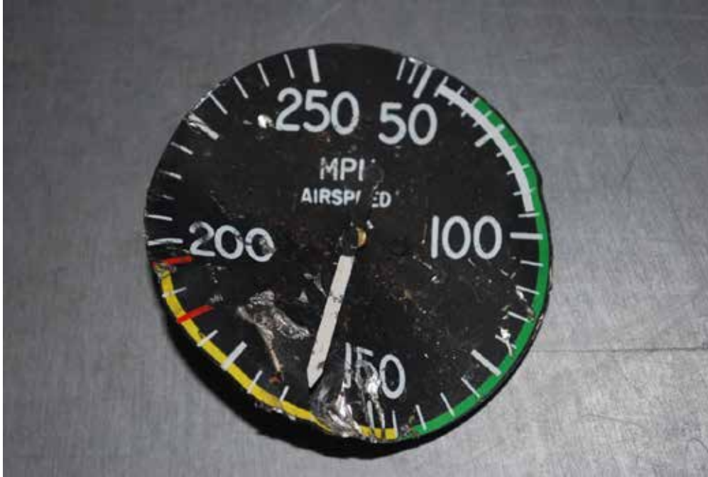
Figure 2. ASI dial removed from accident aircraft
