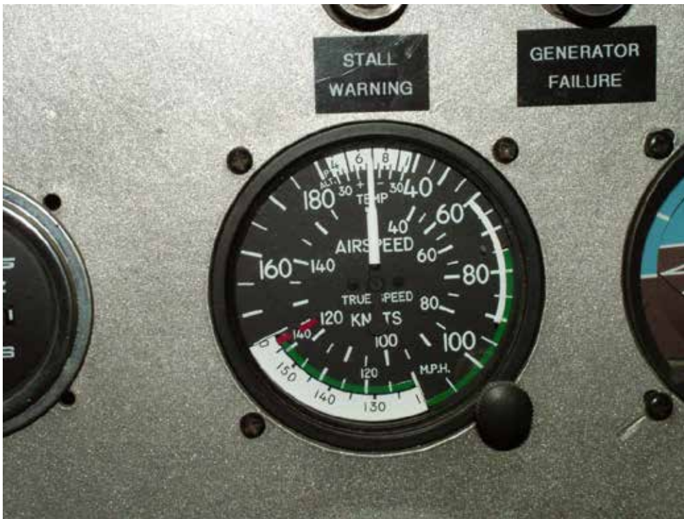
Figure 3. ASI dial on FAR 1505(c) compliant DHC-3T
