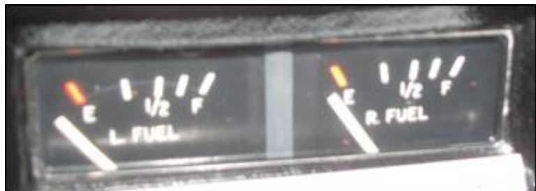
Photo 1. Example of Cessna A185E fuel quantity indicators
