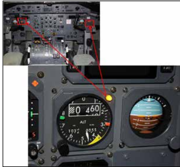
Photo 2. Altitude warning light
