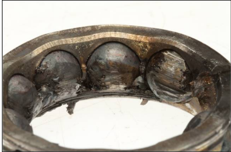
Photo 2. Ball and cage damage
