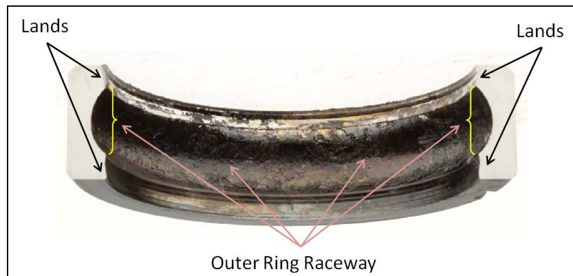
Photo 1. Outer ring raceway showing damaged lands
