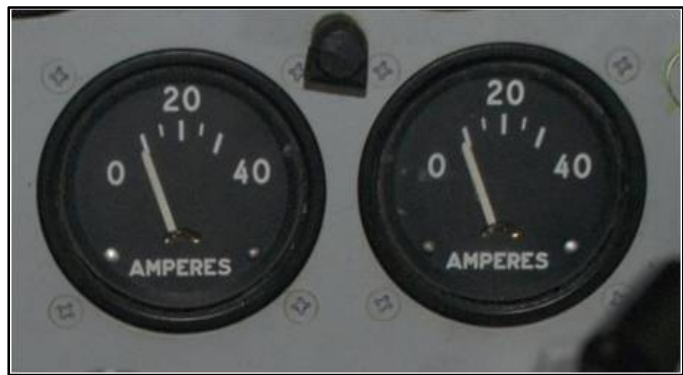
Photo 1. C-FBJA ammeter reading with Generators OFF
