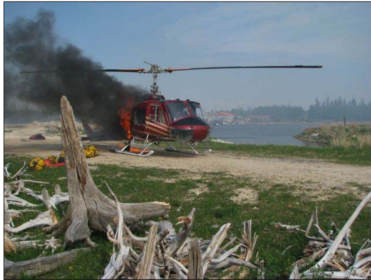
Photo 1. Helicopter showing fire emanating from the engine area.
